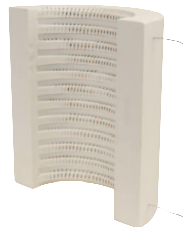
High Temperature (1200°C) Semi-Cylindrical Heater 7" I.D. × 11" O.D. × 12" Long 1600W, 240V
